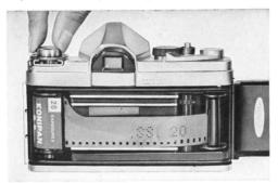
[3] pull out enough film to reach across the film gate. Matching the edge of the film to the flange of the take-up spool, insert film end in the slit of the spool core (take-up spool turn freely, so bring slit into position for easy insertion of film end).
