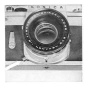
The automatic aperture of the KONICA FS lenses remains at full opening for focusing and sighting, regardless of the pre-selected setting for picturetaking. However, the pre-selected setting can be obtained by pushing the manual aperture lever, so it is possible to see on the focusing screen the degree of sharpness lost in front of and behind the main subject at the aperture size selected for actual exposure.
