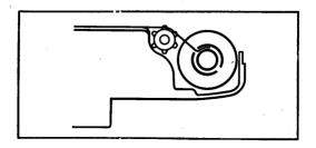
4 Operating the cocking lever while guiding the film perforations onto the sprocket teeth will cause the film to be taken up on the take-up spool.
