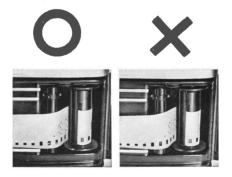
[5] Close backlid, and press shutter button. Turn rewind knob in direction of arrow to take up slack of film
