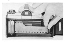
If film end is inserted in the take-up spool slit in the manner shown here, it will easily detach at the end of rewind action.
