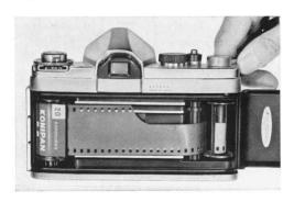
Perforations are fitted onto sprocket teeth
