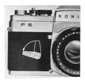
The selftimer mechanism is set by turning the selftimer lever about 70 degrees, either before or after cocking the camera. With the selftimer set, pressing the shutter button will not immediately release the shutter, but will trigger off the selftimer mechanism which, after a delay of about 10 seconds, will actuate the shutter.
