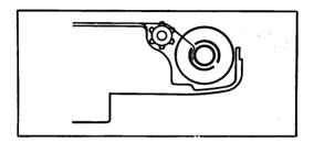
■ If film end happens to be inserted in take-up spool in the manner shown here, it will not slip out of slit at completion of rewind into safety cartridge. In this case, do not force. Open backlid and release film by gently tugging with fingertips.
