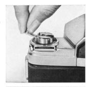
Open backlid, and pull out rewind crank and knob to release safety cartridge for removal.
