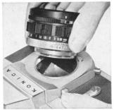
To Attach Lens Match red dots of the lens barrel and camera body, then sinsert lens barrel squarely in the mount. Turn clockwise until the lens catch engages with a click.
