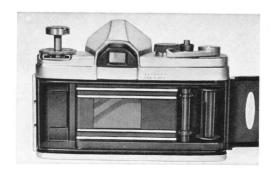
Insert safety cartridge containing unexposed film in the film chamber, and push rewind spindle back into original position, turning it a little to engage spool of safety cartridge.
